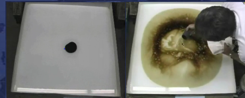
Surfactant contamination of the water surface in a closed system keeps oil from sheening and thereby eliminates dispersion from sheens
