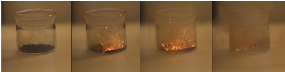
Fig.1. Illustration of the progress of the ambient-temp. reaction between \text{AgF}_2 and \text{SiCl}_4 .
